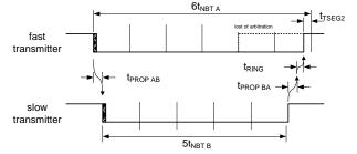
$t_{PROP AB RD} + t_{PROP BA RD} \le t_{NBT} - t_{TSEG2} - (19t_{NBT} - t_{TSEG2}) df$
