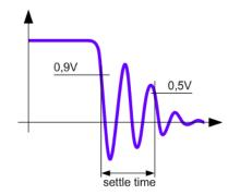
The settle time test does not consider any delays or baud rate drifts.
