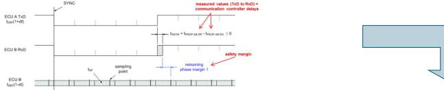
$$\frac{t_{ASYM}}{t_{DBT}} < \left(5 + \frac{t_{SPB}}{t_{DBT}} - \frac{t_{TQB}}{t_{DBT}}\right) (1 - dt_B) - 5(1 + dt_A) - \frac{t_{RPM1}}{t_{DBT}}$$
