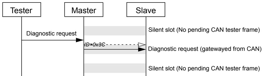
Figure 5.1: Gatewaying of CAN messages to LIN.
