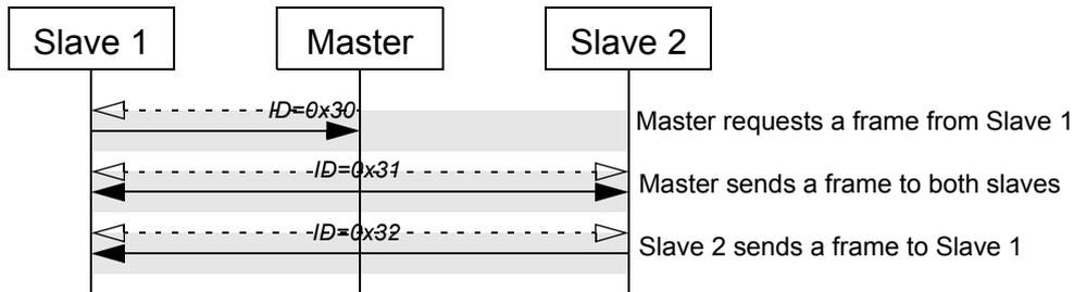
Figure 2.9: Three unconditional frame transfers.
