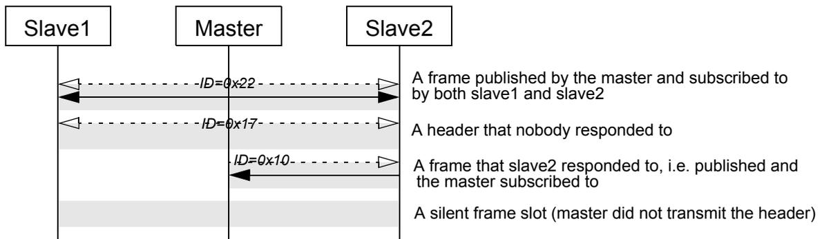
Figure 2.19: Frame sequence example.
