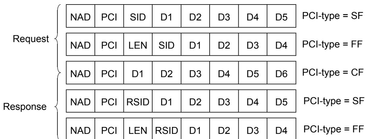
Figure 3.2: PDUs supported by the LIN transport layer.
