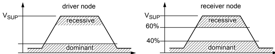
*Figure 6.4: Voltage Levels on the Bus Line*
