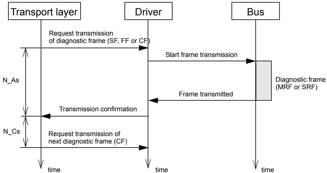
Figure 3.3: Transport layer timing on transmitter side
