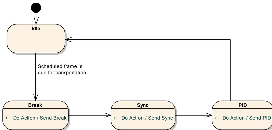
Figure 2.13: Complete state machine for the master task.
