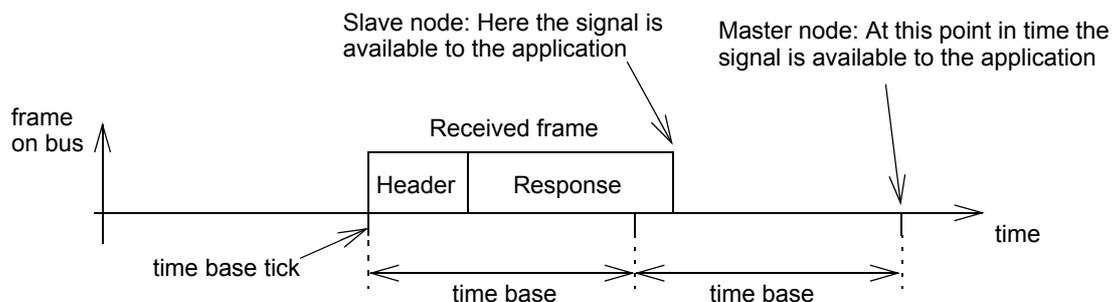
Figure 2.1: Timing of signal reception
