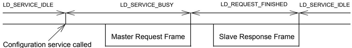
Figure 7.2: Successful configuration request and configuration response
