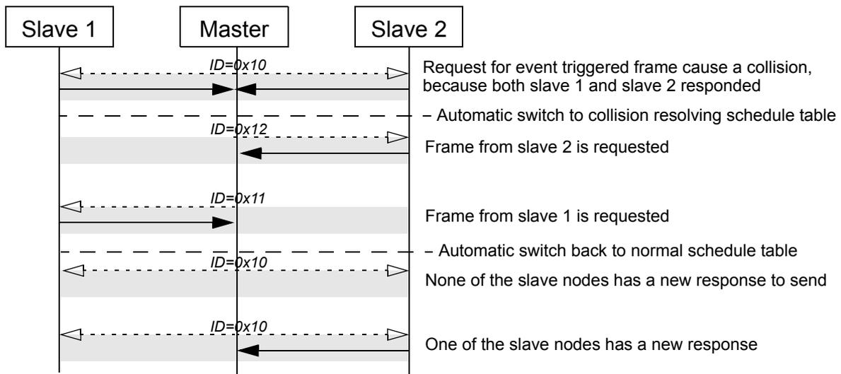
Figure 2.10: Event-triggered frame example.
