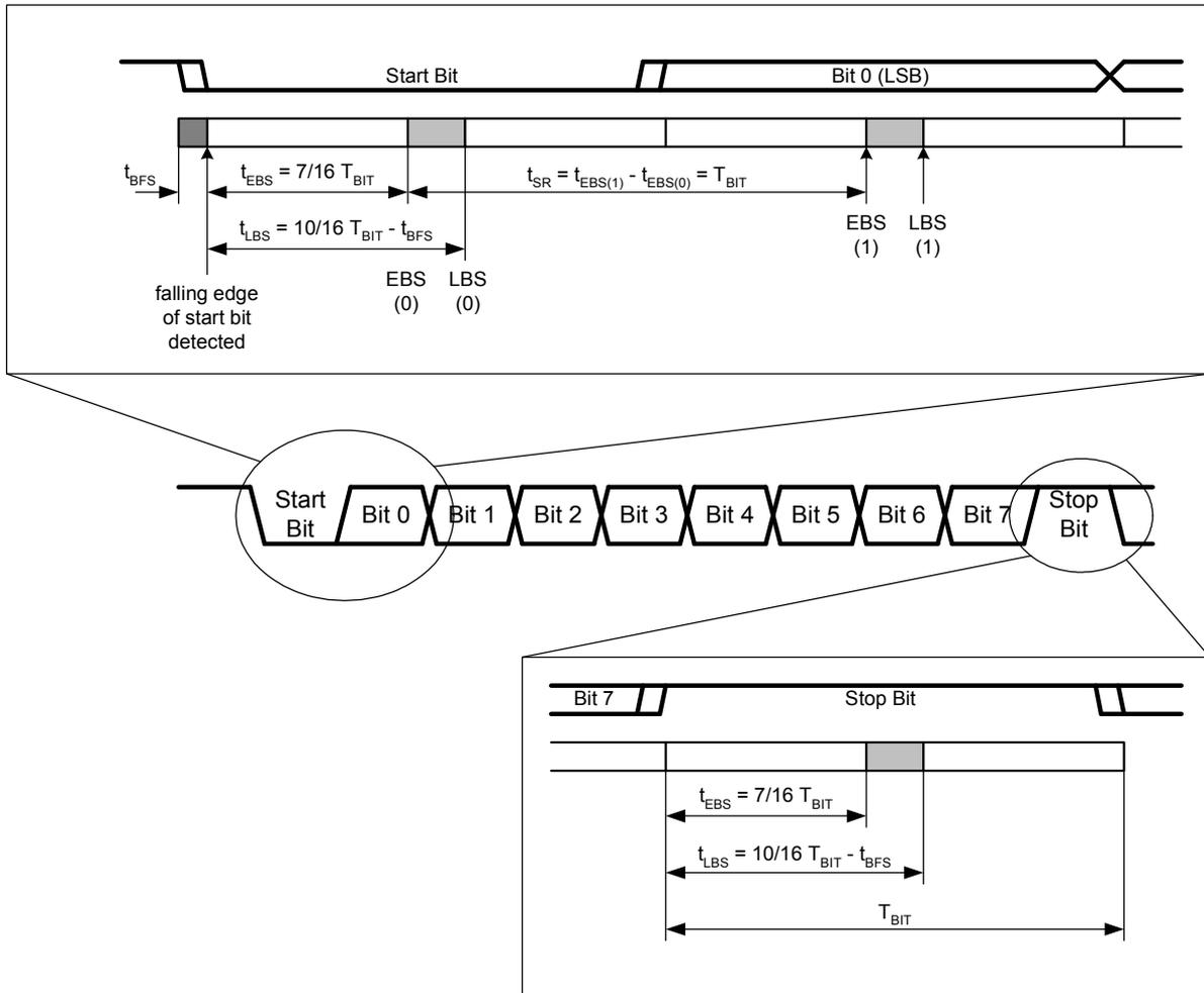
Figure 6.2: Bit Sample Timing
