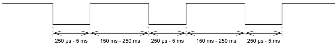
Figure 2.17: One block of wake up signals
