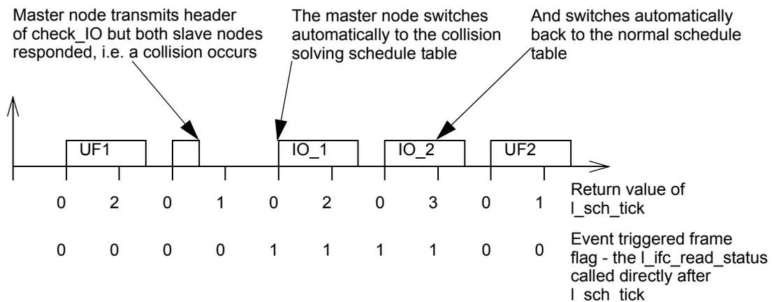
Figure 7.1: Event triggered frame collision solving example
