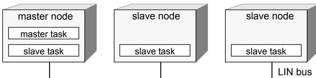
The master task decides when and which frame shall be transferred on the bus. The slave tasks provide the data transported by each frame.
