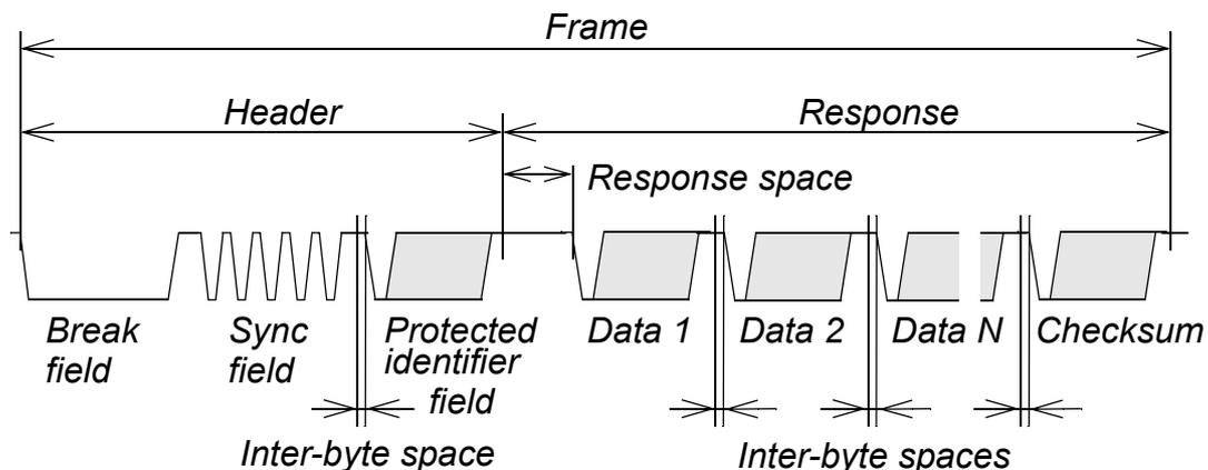
Figure 2.3: The structure of a frame.
