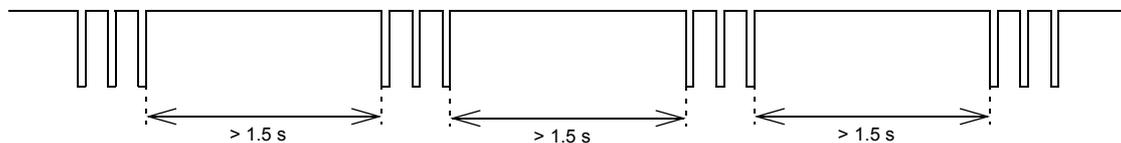
Figure 2.18: Wake up signals over long time
