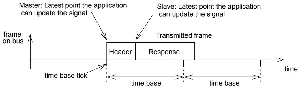
*Figure 2.2: Timing of signal transmission*
