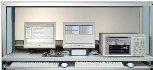
Figure 5: C&S CAN / CAN FD Automated Test System.
